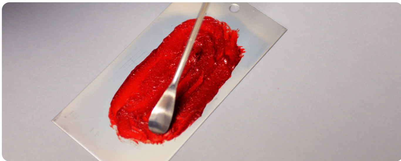
An example process residue sample is coated on a stainless steel coupon for a PACE Cleaning Evaluation
